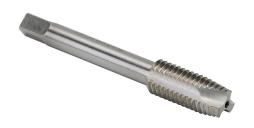
RUKO hand tap, M10 x 1.50 coarse, square shank per DIN 10, high-speed steel (HSS), bright finish.
