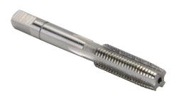
RUKO hand tap, M6 x 1.0 coarse, square shank per DIN 10, high-speed steel (HSS), bright finish.
