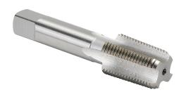
RUKO hand tap, 3/8-18 NPT, square shank per DIN 10, high-speed steel (HSS), bright finish.
