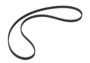
SureMotion timing belt, 1/5in XL pitch, 1/4in wide, 115 tooth, 23in pitch length (circumference), neoprene, fiberglass reinforced.
