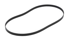
SureMotion timing belt, 0.08in MXL pitch, 1/4in wide, 230 tooth, 18.4in pitch length (circumference), polyurethane, polyester reinforced. Package of 3.
