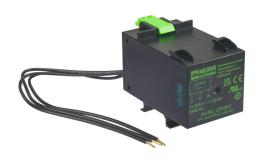
Murrelektronik motor surge suppressor, resistor-capacitor, 575 VAC, 3-phase, 50/60 Hz, 7.5 kW, pigtail with end ferrule, 35mm DIN rail mount.
