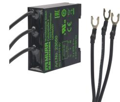
Murrelektronik motor surge suppressor, resistor-capacitor, 575 VAC, 3-phase, 50/60 Hz, 4 kW, pigtail with spade connectors, adhesive foil mount.
