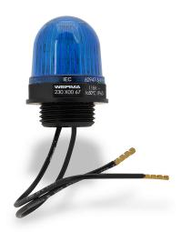
WERMA LED industrial signal beacon, 29mm, blue, permanent, IP65, M20  $\times$  1.5 threaded base mount, 115 VAC.
