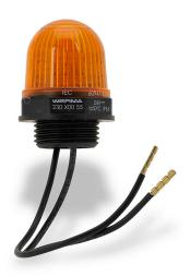
WERMA LED industrial signal beacon, 29mm, yellow, permanent, IP65, M20 x 1.5 threaded base mount, 24 VDC.
