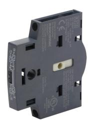
Socomec auxiliary contact, left or right side mount, (1) N.O. pre-break/(1) N.C. contact(s), 6A @ 120 VAC. For use with SIRCO M and SIRCO M Compact 16-100A switch bodies.
