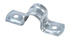
Minerallac 2-hole conduit mount strap, standard duty, UL Type UL 1565. Package of 100. For use with 3/8in LFMC, 1/2in EMT, 6 AWG.
