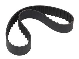
SureMotion timing belt, 3/8in L pitch, 1in wide, 60 tooth, 22.5in pitch length (circumference), neoprene, fiberglass reinforced.
