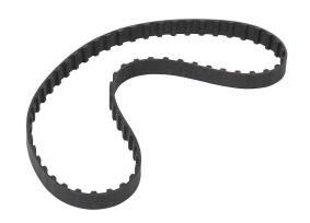
SureMotion timing belt, 3/8in L pitch, 1/2in wide, 60 tooth, 22.5in pitch length (circumference), neoprene, fiberglass reinforced.
