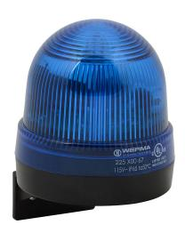
WERMA Xenon tube industrial signal beacon, 75mm, blue, flashing strobe (0.75 Hz flash frequency), IP65, bracket mount, 115 VAC.
