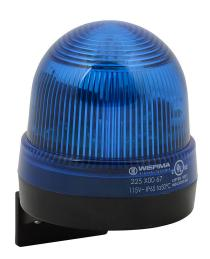
WERMA Xenon tube industrial signal beacon, 75mm, blue, flashing strobe (0.75 Hz flash frequency), IP65, bracket mount, 115 VAC.
