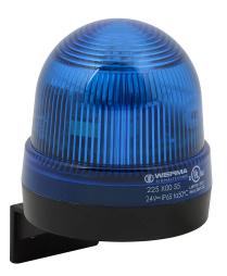
WERMA Xenon tube industrial signal beacon, 75mm, blue, flashing strobe (0.75 Hz flash frequency), IP65, bracket mount, 24 VDC.
