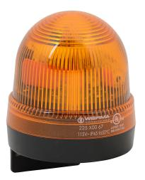
WERMA Xenon tube industrial signal beacon, 75mm, yellow, flashing strobe (0.75 Hz flash frequency), IP65, bracket mount, 115 VAC.
