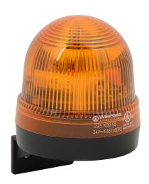
WERMA Xenon tube industrial signal beacon, 75mm, yellow, flashing strobe (0.75 Hz flash frequency), IP65, bracket mount, 24 VDC.
