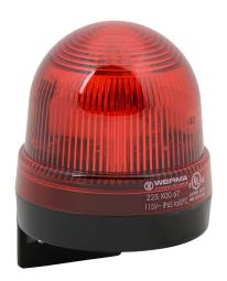
WERMA Xenon tube industrial signal beacon, 75mm, red, flashing strobe (0.75 Hz flash frequency), IP65, bracket mount, 115 VAC.
