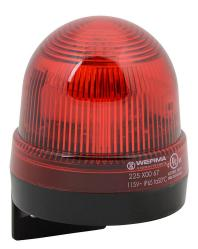
WERMA Xenon tube industrial signal beacon, 75mm, red, flashing strobe (0.75 Hz flash frequency), IP65, bracket mount, 115 VAC.
