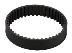
SureMotion timing belt, 5mm 5M pitch, 15mm wide, 45 tooth, 225mm pitch length (circumference), neoprene, fiberglass reinforced.
