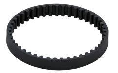
SureMotion timing belt, 5mm 5M pitch, 9mm wide, 45 tooth, 225mm pitch length (circumference), neoprene, fiberglass reinforced.
