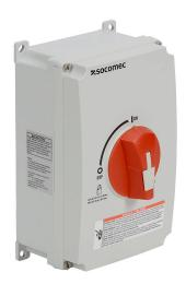
Socomec SIRCO M series rotary enclosed disconnect switch, load break capable, 3-pole, 600 VAC, 60A, 50kA SCCR, wall mount, UL 508 rated,  $4.94 \times 8.27 \times 4.37$  in housing.
