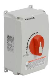
Socomec SIRCO M series rotary enclosed disconnect switch, load break capable, 3-pole, 600 VAC, 30A, 65kA SCCR, wall mount, UL 508 rated, 4.94 x 8.27 x 4.37in housing.
