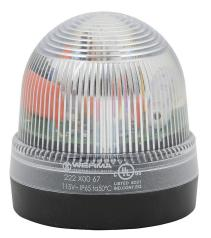
WERMA Xenon tube industrial signal beacon, 75mm, clear/white, flashing strobe (0.75 Hz flash frequency), IP65, base mount, 115 VAC.
