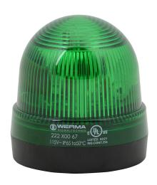
WERMA Xenon tube industrial signal beacon, 75mm, green, flashing strobe (0.75 Hz flash frequency), IP65, base mount, 115 VAC.
