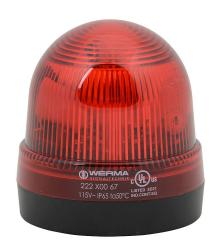
WERMA Xenon tube industrial signal beacon, 75mm, red, flashing strobe (0.75 Hz flash frequency), IP65, base mount, 115 VAC.
