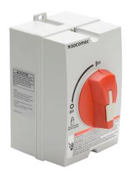
Socomec SIRCO M series rotary enclosed disconnect switch, load break capable, 3-pole, 600 VAC, 30A, 65kA SCCR, wall mount, UL 508 rated,  $3.9 \times 6.38 \times 4.37$ in housing.
