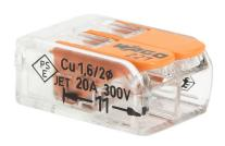
WAGO 221 series splicing connector, lever, side-entry, 2 openings, copper conductor, 24-12 AWG solid, 24-12 AWG stranded, 20A, 600V, polycarbonate housing, transparent/orange. Package of 100.
