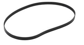
SureMotion timing belt, 0.08in MXL pitch, 1/4in wide, 220 tooth, 17.6in pitch length (circumference), polyurethane, polyester reinforced. Package of 3.
