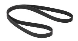
SureMotion timing belt, 0.08in MXL pitch, 1/4in wide, 220 tooth, 17.6in pitch length (circumference), neoprene, fiberglass reinforced. Package of 3.
