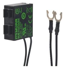
Murrelektronik universal surge suppressor, resistor-capacitor, 127-240 VAC/VDC, 1-phase, 0-60Hz, 15W, pigtail with spade connectors, contactor mount.
