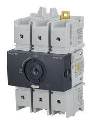
Socomec SIRCO M Compact series rotary disconnect switch, load break capable, 3-pole, 600 VAC, 60A, 100kA SCCR, DIN rail or panel mount, UL 98 rated, front or side operated, accepts 5 x 5mm size shaft.
