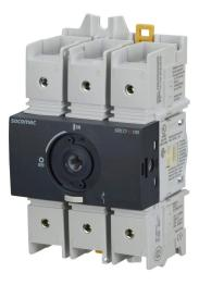
Socomec SIRCO M Compact series rotary disconnect switch, load break capable, 3-pole, 600 VAC, 100A, 100kA SCCR, DIN rail or panel mount, UL 98 rated, front or side operated, accepts 5 x 5mm size shaft.
