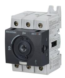
Socomec SIRCO M series rotary disconnect switch, load break capable, 3-pole, 600 VAC, 80A, 65kA SCCR, DIN rail or panel mount, UL 508 rated, front or side operated, accepts 5 x 5mm size shaft.
