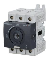
Socomec SIRCO M series rotary disconnect switch, load break capable, 3-pole, 600 VAC, 63A, 65kA SCCR, DIN rail or panel mount, UL 508 rated, front or side operated, accepts 5 x 5mm size shaft.
