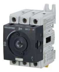
Socomec SIRCO M series rotary disconnect switch, load break capable, 3-pole, 600 VAC, 40A, 65kA SCCR, DIN rail or panel mount, UL 508 rated, front or side operated, accepts 5 x 5mm size shaft.
