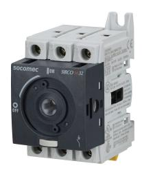
Socomec SIRCO M series rotary disconnect switch, load break capable, 3-pole, 600 VAC, 32A, 65kA SCCR, DIN rail or panel mount, UL 508 rated, front or side operated, accepts 5 x 5mm size shaft.
