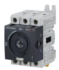
Socomec SIRCO M series rotary disconnect switch, load break capable, 3-pole, 600 VAC, 25A, 65kA SCCR, DIN rail or panel mount, UL 508 rated, front or side operated, accepts 5 x 5mm size shaft.
