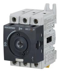
Socomec SIRCO M series rotary disconnect switch, load break capable, 3-pole, 600 VAC, 20A, 65kA SCCR, DIN rail or panel mount, UL 508 rated, front or side operated, accepts 5 x 5mm size shaft.
