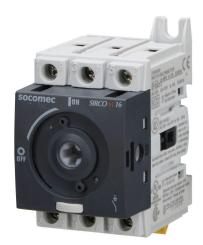
Socomec SIRCO M series rotary disconnect switch, load break capable, 3-pole, 600 VAC, 16A, 65kA SCCR, DIN rail or panel mount, UL 508 rated, front or side operated, accepts 5 x 5mm size shaft.
