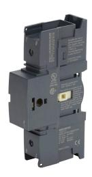
Socomec fourth pole module, 600 VAC, 100A, load break capable, 100kA SCCR, UL 98 rated. For use with SIRCO M Compact 30-100A switch bodies.
