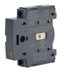
Socomec fourth pole module, 600 VAC, 32A, load break capable, 65kA SCCR, UL 508 rated. For use with SIRCO M 32A switch body.
