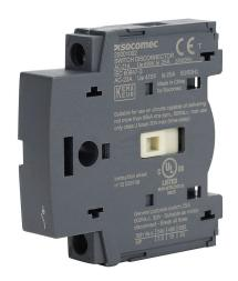
Socomec fourth pole module, 600 VAC, 25A, load break capable, 65kA SCCR, UL 508 rated. For use with SIRCO M 25A switch body.
