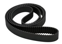
SureMotion timing belt, 8mm 8M pitch, 30mm wide, 275 tooth, 2200mm pitch length (circumference), neoprene, fiberglass reinforced.
