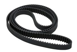
SureMotion timing belt, 8mm 8M pitch, 20mm wide, 275 tooth, 2200mm pitch length (circumference), neoprene, fiberglass reinforced.
