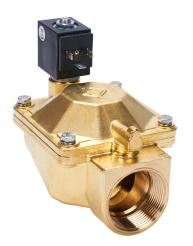
ODE potable water solenoid valve, 2-port (2-way), 2-position, N.C., lead-free brass body, 1-1/2in female NPT inlet(s), 1-1/2in female NPT outlet(s), Cv=36, 24 VDC operating voltage, 11W, NSF/ANSI 169.
