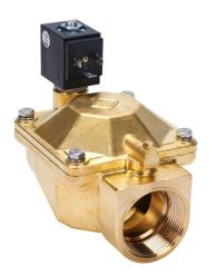
ODE potable water solenoid valve, 2-port (2-way), 2-position, N.C., lead-free brass body, 1-1/2in female NPT inlet(s), 1-1/2in female NPT outlet(s), Cv=36, 120 VAC (60Hz)/110 VAC (50Hz) operating voltage, 15 VA, NSF/ANSI 169.
