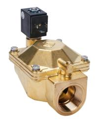
ODE potable water solenoid valve, 2-port (2-way), 2-position, N.C., lead-free brass body, 1-1/4in female NPT inlet(s), 1-1/4in female NPT outlet(s), Cv=28, 24 VDC operating voltage, 11W.
