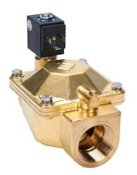
ODE potable water solenoid valve, 2-port (2-way), 2-position, N.C., lead-free brass body, 1-1/4in female NPT inlet(s), 1-1/4in female NPT outlet(s), Cv=28, 120 VAC (60Hz)/110 VAC (50Hz) operating voltage, 15 VA, NSF/ANSI 169.
