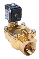
ODE potable water solenoid valve, 2-port (2-way), 2-position, N.C., lead-free brass body, 1in female NPT inlet(s), 1in female NPT outlet(s), Cv=14, 24 VDC operating voltage, 11W.
