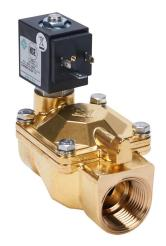
ODE potable water solenoid valve, 2-port (2-way), 2-position, N.C., lead-free brass body, 1in female NPT inlet(s), 1in female NPT outlet(s), Cv=14, 120 VAC (60Hz)/110 VAC (50Hz) operating voltage, 15 VA, NSF/ANSI 61.
